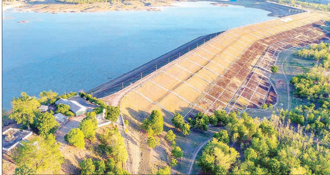
An aerial view of Mann Chaung Dam. Mann Chaung Dam can store water approximately to 83,250 acre-feet and will supply adequate irrigation to 18,760 acres of summer crops in Minbu Township, according to Irrigation and Water Utilization Management Department. PHOTO: NAY THIT
