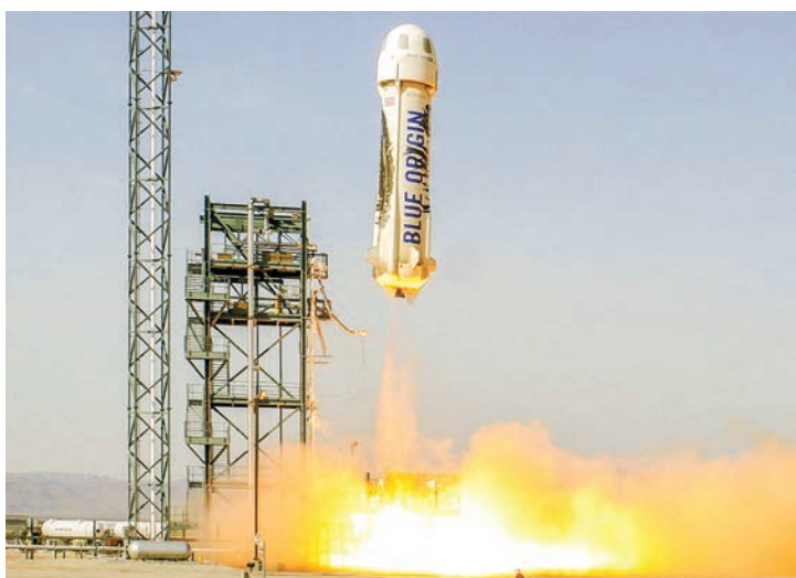
Blue Origin's New Shepard rocket burns liquid hydrogen and liquid oxygen, which combusts as water vapour. PHOTO: MRTEGDIF/TWITTER/AFP
