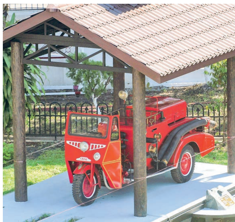
Daihatsu three-wheeled car fire engine with Centrifugal Pump was for narrow roads and they are mostly used in the rural areas across Myanmar.
